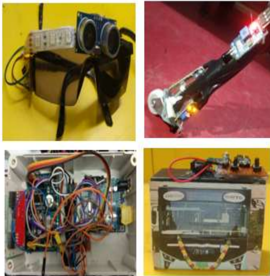
Fig 2: Snapshot of model of Ultrasonic bifocal for visually impaired person
